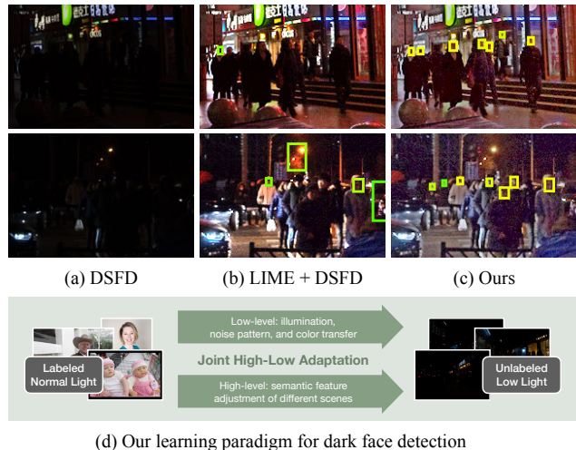
Figure 1. Dark face detection visual results and our learning paradigm. Compared with the result of DSFD [26] on original low light images and the enhanced version by LIME [16], our method can better recognize the faces in dark scenarios.
